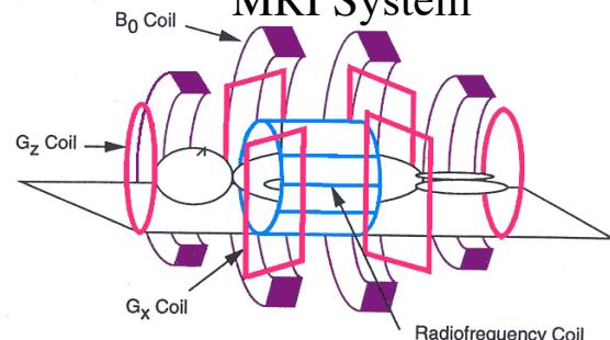
Simplified Drawing of Basic Instrumentation.
